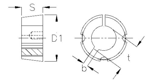
$\begin{array}{lll} b & = 5 \\ Bore & = 14 \\ Bush type & = 1310 \\ D1 & = 50,5 \\ S & = 25,4 \\ Screw size & = 3/8 \times 5/8" \\ t & = 16.3 \end{array}$
